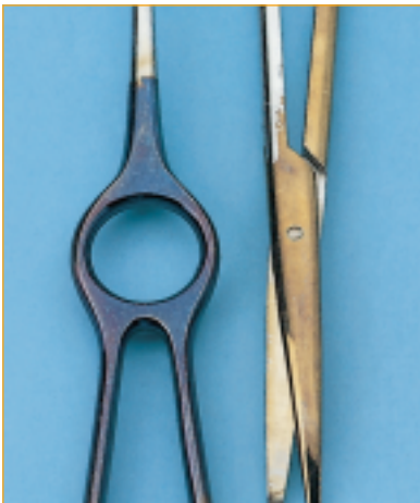
Discoloration of instruments. Cause: insufficient rinsing
