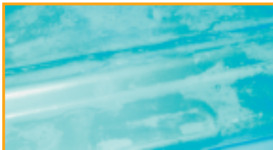
attacked Eloxal (anodized aluminum)
