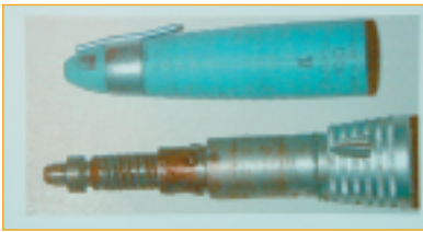
Blood residues on a handle Cause: insufficient cleaning
