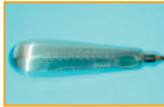
Stained instruments Cause: Drying water
