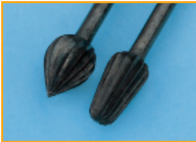
Corrosion on burs Cause: Reprocessing of disposable instruments
