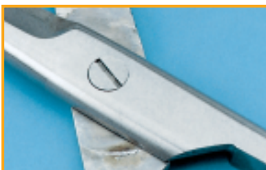
Corrosion on scissors. Cause of corrosion: lack of maintenance, no oil
